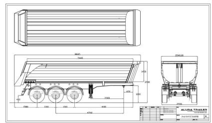
**Body:** Tipper body will be single steel plate with the pressing. Tipper body welding will be MIG welding method. Body floor will be 5 mm ST 52-3 quality steel. Side of the Tipper body will be 4 mm ST 52-3 quality steel. Support steel of the body will be 4 mm ST 52-3 quality steel. All the welding will be MIG and synergic MIG welding with protective mixed argon gas.
